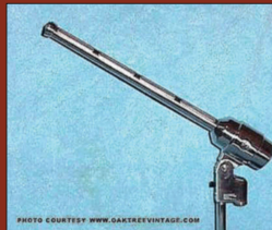
Figure 6.6 Early "shotgun" mic. Clever mechanical placement of baffles and pickup elements made for a mic that was highly directional.
