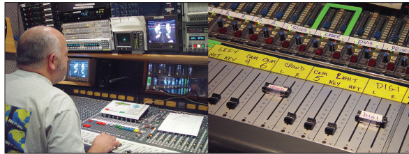
Figure 6.8 Today's boards are so flexible that most likely no two AIs would organize and mix a show the same way. Some boards have multiple sets of faders, and allow faders to control different sources with the push of a button. Most high-end "boards" let you assign often-used sources to close faders, and the "set once and forget" sources, often part of a sub-mix, to faders not as conveniently located.
