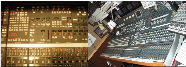
Figure 6.7 Audio consoles historically doubled as the audio mixer also, as the audio actually passed through the operator's console. Today's mixers, especially digital ones, have extremely high-powered Digital signal processing occurring. As a result, many mixers today are organized like video switchers, with one operations console, which controls the frame that does the processing and mixing of audio, per input from the audio console. (Source: Marty Etbeck)
