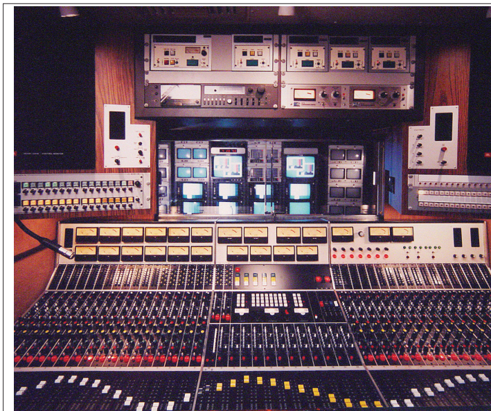
Figure 6.4 By the '80s audio mixers closely resembled many of today's consoles, as this mixer on a network truck attests. (Source: A.F. Associates)
